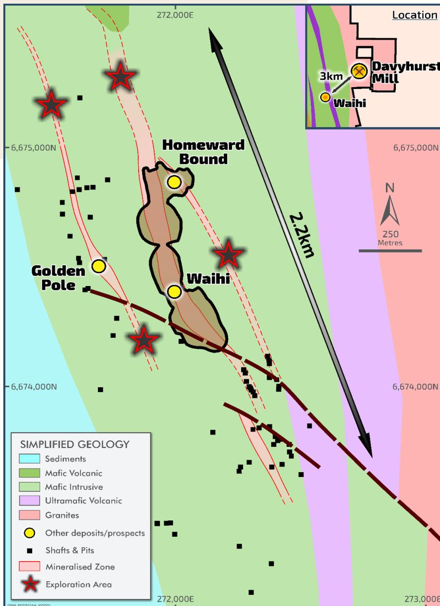
Figure 1 – Waihi overview plan showing mineralised lodes within the Main Mining Area, historic workings and proximity to Davyhurst Mill.
