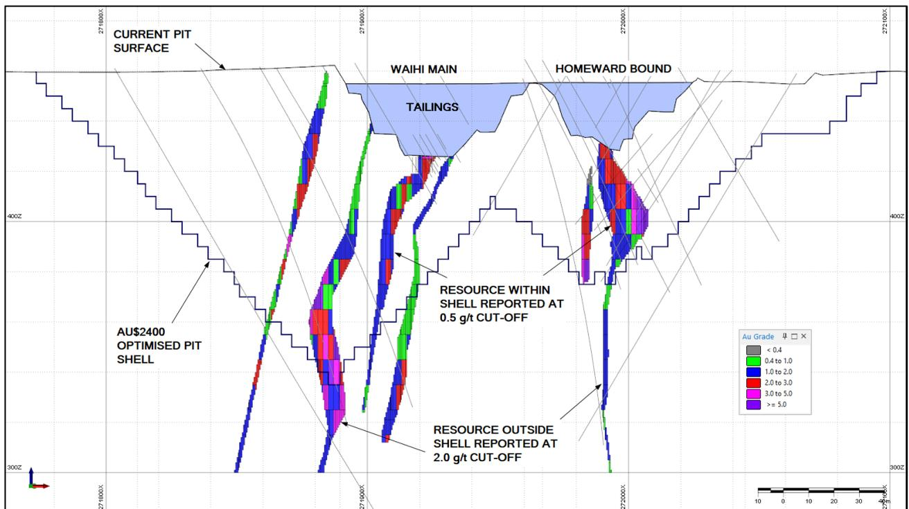
Figure 4 – Oblique Cross Section (6674830mN) showing resource and AU\$2400 per ounce pit shell
