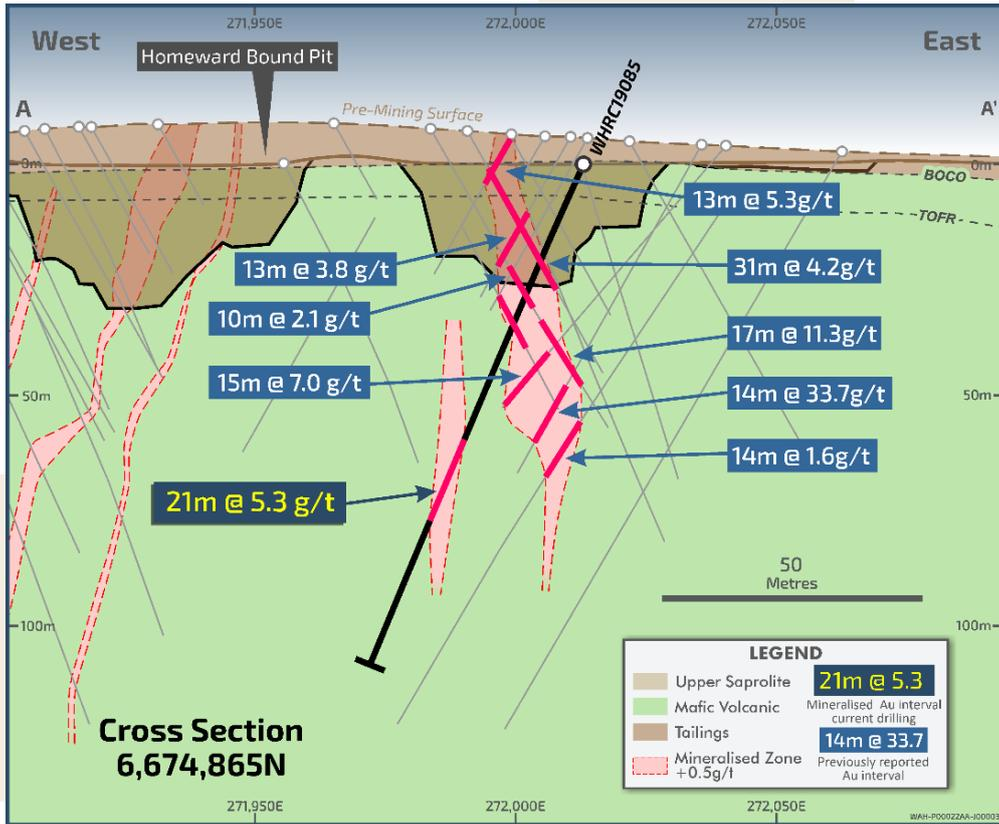
Figure 2 – Cross Section highlighting results from recent drilling
