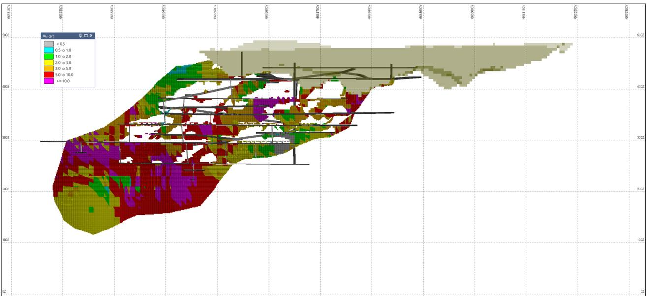
Figure 5 – Long section view looking west of the Callion Main Lode block model below the optimised \$2,400/oz pit shell. Existing underground development and stoping voids are also highlighted
