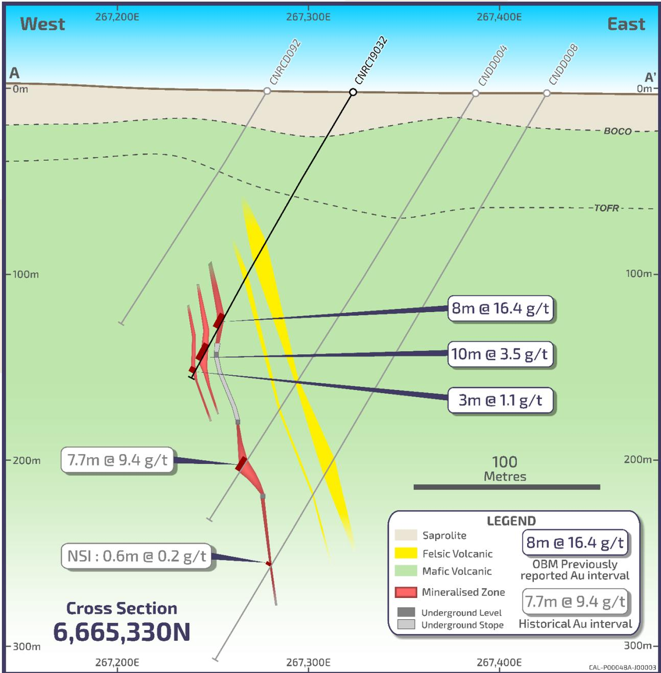
Figure 3 – Cross Section highlighting results from recent drilling relative to old underground stopes
