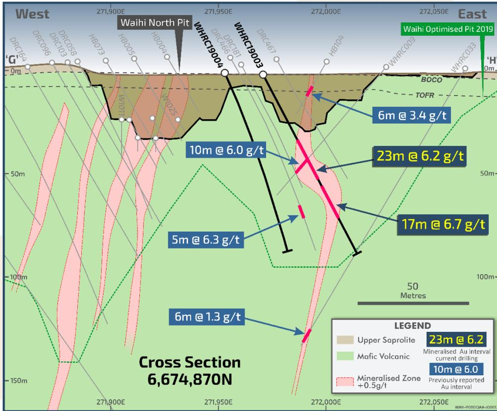
Figure 3 – Cross Section of recent drilling
