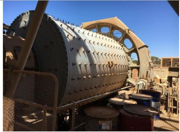
**Milling Circuit – Ball Mill**
