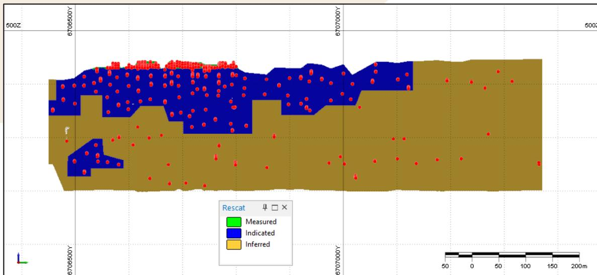
Figure 4 Riverina Main Lode West Long Section (looking west) showing classification and sample locations
