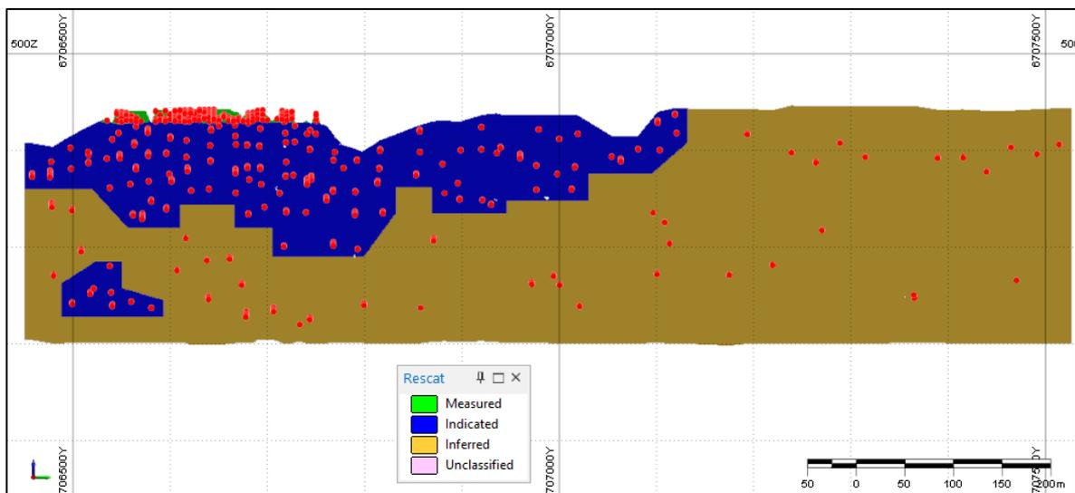
Figure 5 Isometric View (looking down towards the NE) showing classification of mineralised lodes
